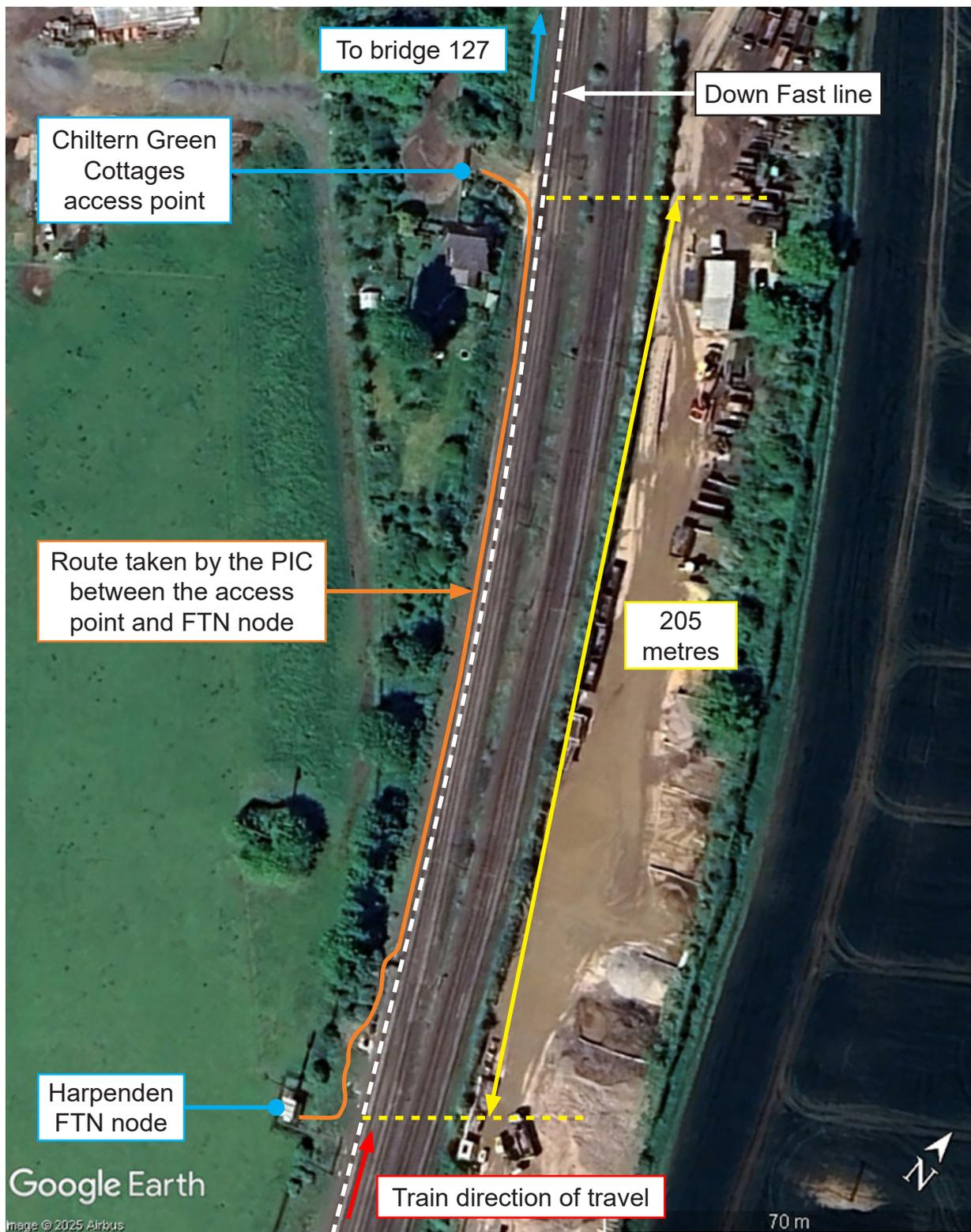
Figure 8: The route taken between the access point at Chiltern Green Cottages and the FTN node (courtesy of Google with RAIB annotations).
