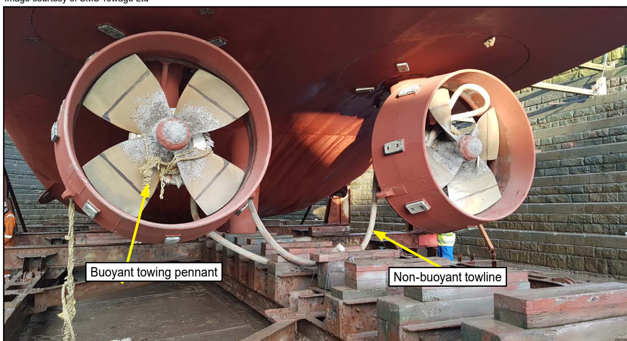
Figure 7: Yeoman 's propellers fouled by Svitzer Josephine 's towline
