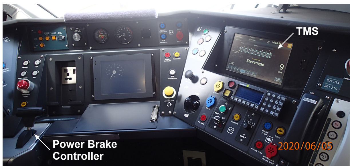
Figure 4: Class 800 cab layout showing TMS and power brake controller
