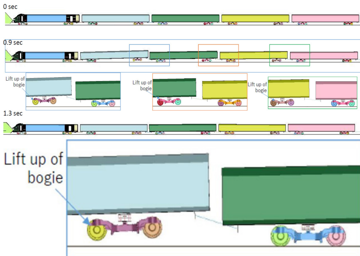
Figure 13: Output from collision and derailment simulation – sequence of events (courtesy of Hitachi)
