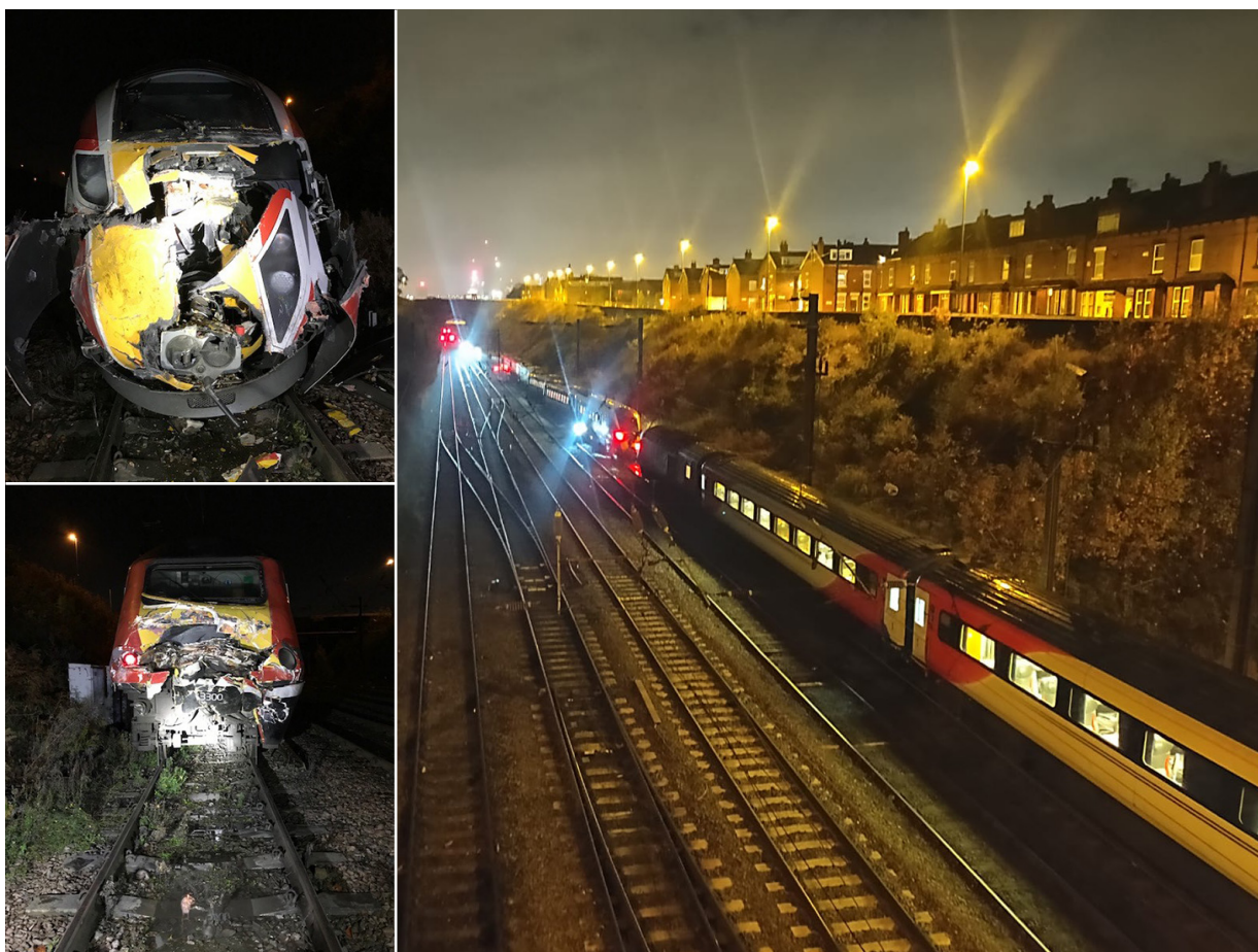
Figure 2: The class 800 train (top) and HST set (bottom) involved in the accident and the crash scene to the right (images courtesy of Network Rail)
