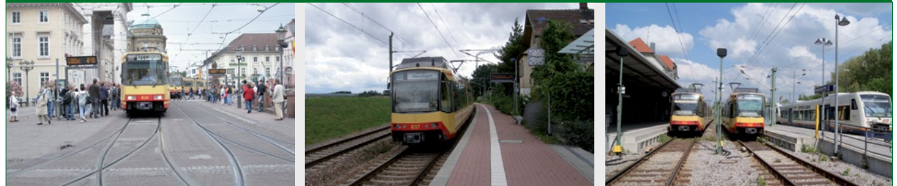
Figure 4.2 – Photographs of tram trains in Karlsruhe (left to right) on an on street tramway, in segregated operation, and on heavy rail
