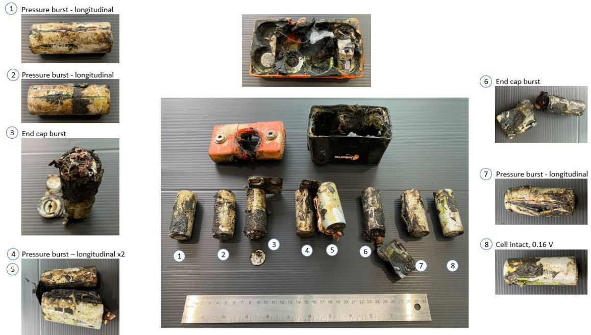
Figure 4 Damaged parts of the battery
