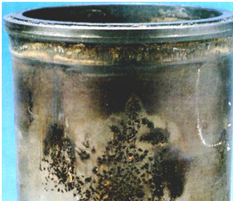
Figure 1. Severely Eroded liner
