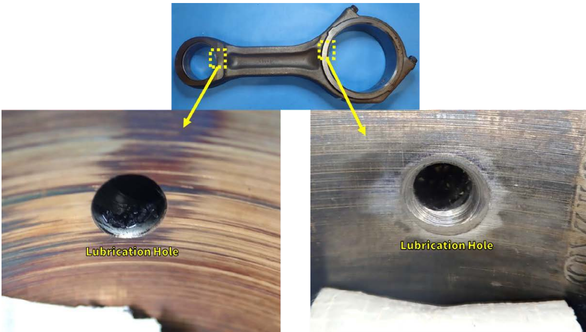
FIGURE 2. Representative photographs of the lubrication channel openings in the subject connecting rod. Particles were visible in both openings.
