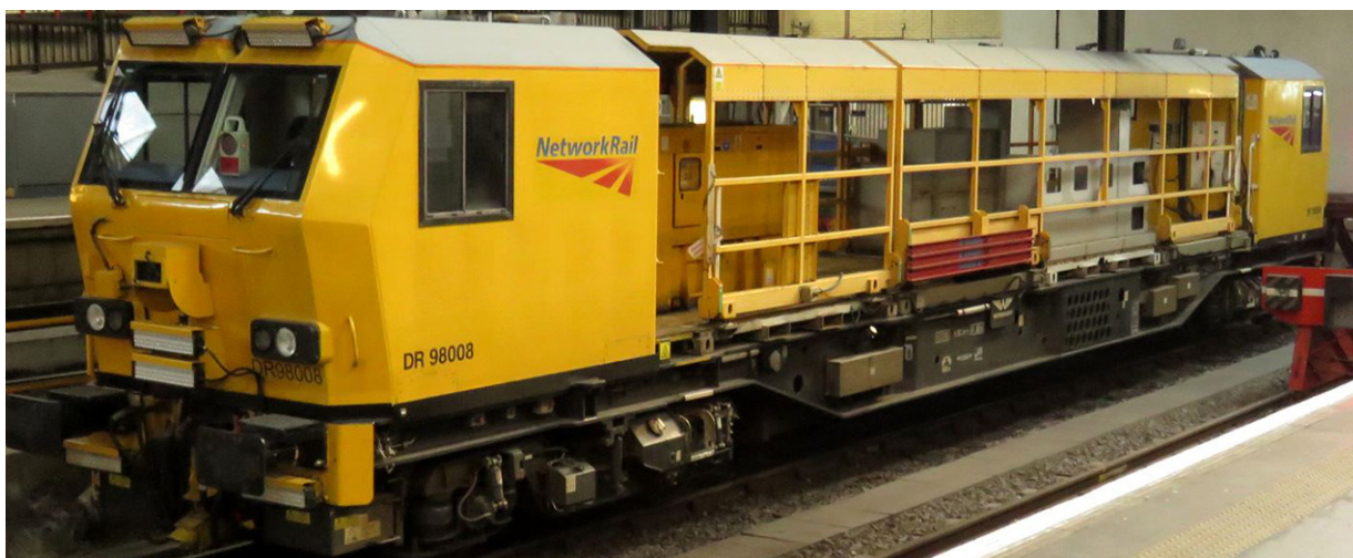
Figure 18: Network Rail's MPV based track recording vehicle (image courtesy of Brian Creasey)
