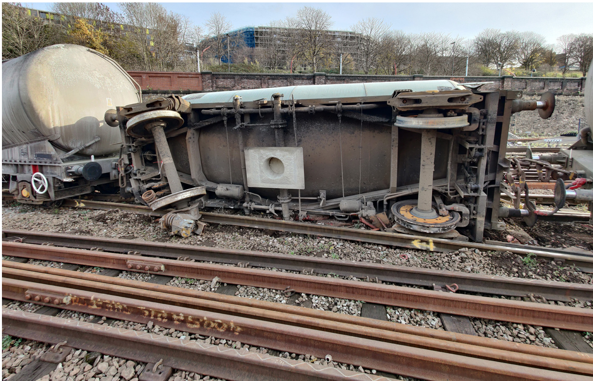
Figure 3: Wagon BCC10756 toppled on its side
