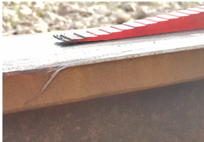
Figure 8: Wheel mark on the inside edge of the right-hand rail showing the first drop-in at the point of derailment (the red step gauge is only present to indicate the point of derailment)
