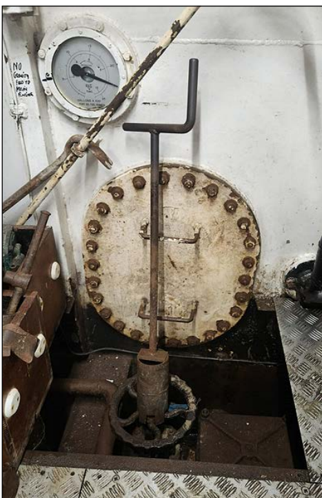
Figure 4: Example of portable extension spindle fitted to the sea inlet valve below the engine room floor plate
