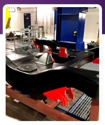
"Replacing steel with recycled carbon fibre to produce a rail bogie is a world first, so it is a hugely exciting and rewarding project to be part of. We hope to make recycled carbon not only an attractive option for the rail industry in terms of weight reduction, but also to eliminate waste and drive down cost." **Frazer Barnes, Managing Director of ELG Carbon Fibre (now Green 2 Carbon)**
