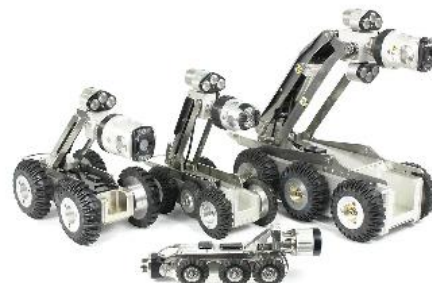
Source: Minicam Ltd, 2022. Image shows robots designed to inspect and maintain sewers.
