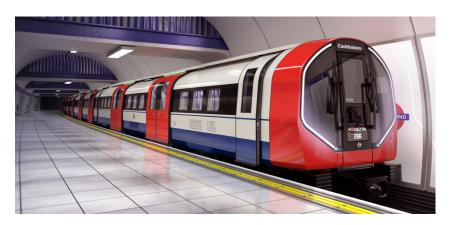
The trains are part of Siemens Mobility's Inspiro family. They boast a 10 per cent capacity increase thanks to an innovative articulated design that reduces the number of bogies required per full length train whilst maximising the available interior space – important in the space-constrained Tube environment. This articulation reduces track damage and has the additional benefit of a smoother and quieter ride for passengers.
