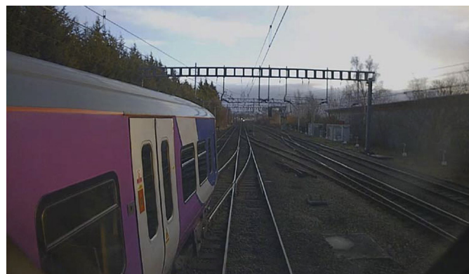
Figure 6: Forward facing camera view of the near miss, taken from the train on the up fast line and showing the train on the up slow line passing over the crossover immediately ahead (image courtesy of CrossCountry trains)
