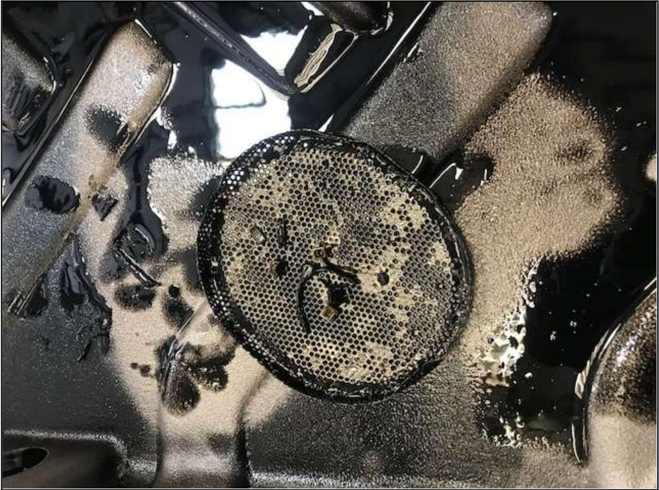
**Figure 29:** Debris found in engine sump pan and lubricating oil strainer
