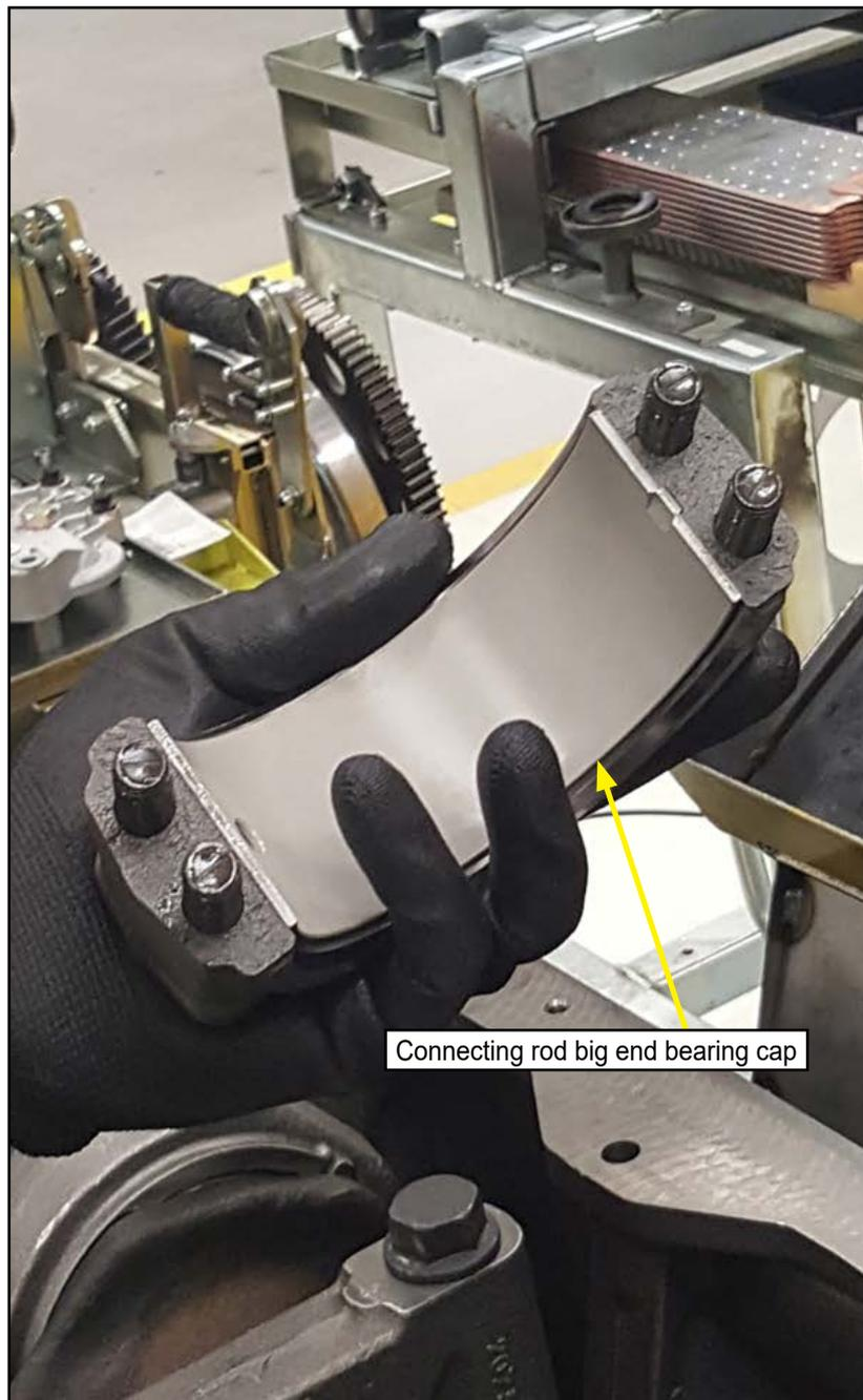
**Figure 7:** D16 MH engine connecting rod installation
