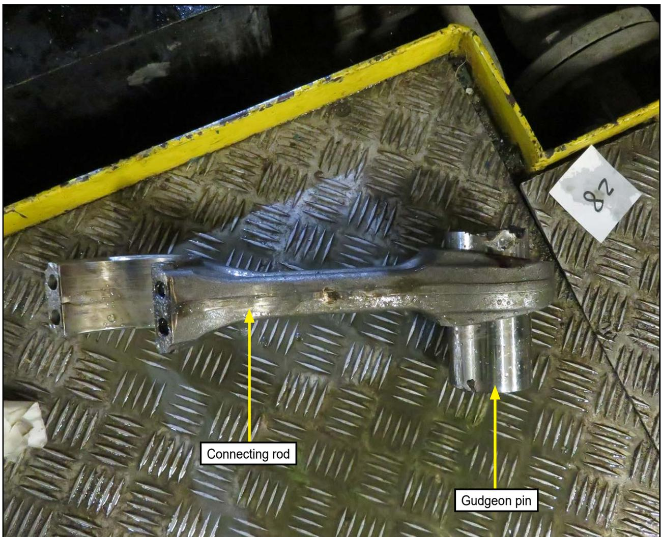
**Figure 5:** ME4 number four connecting rod and gudgeon pin
