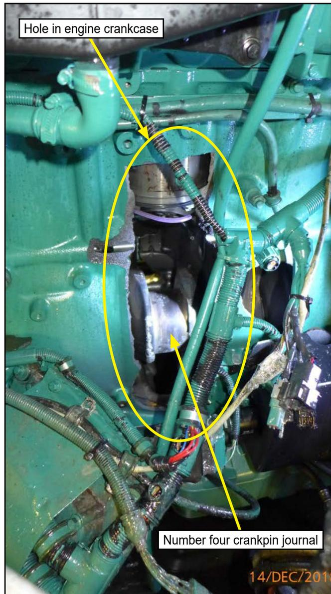
**Figure 6:** Hole in ME4 crankcase/engine block, showing number four crankpin journal
