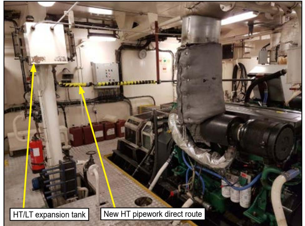
**Figure 16:** Modified cooling system high temperature circuit pipework
