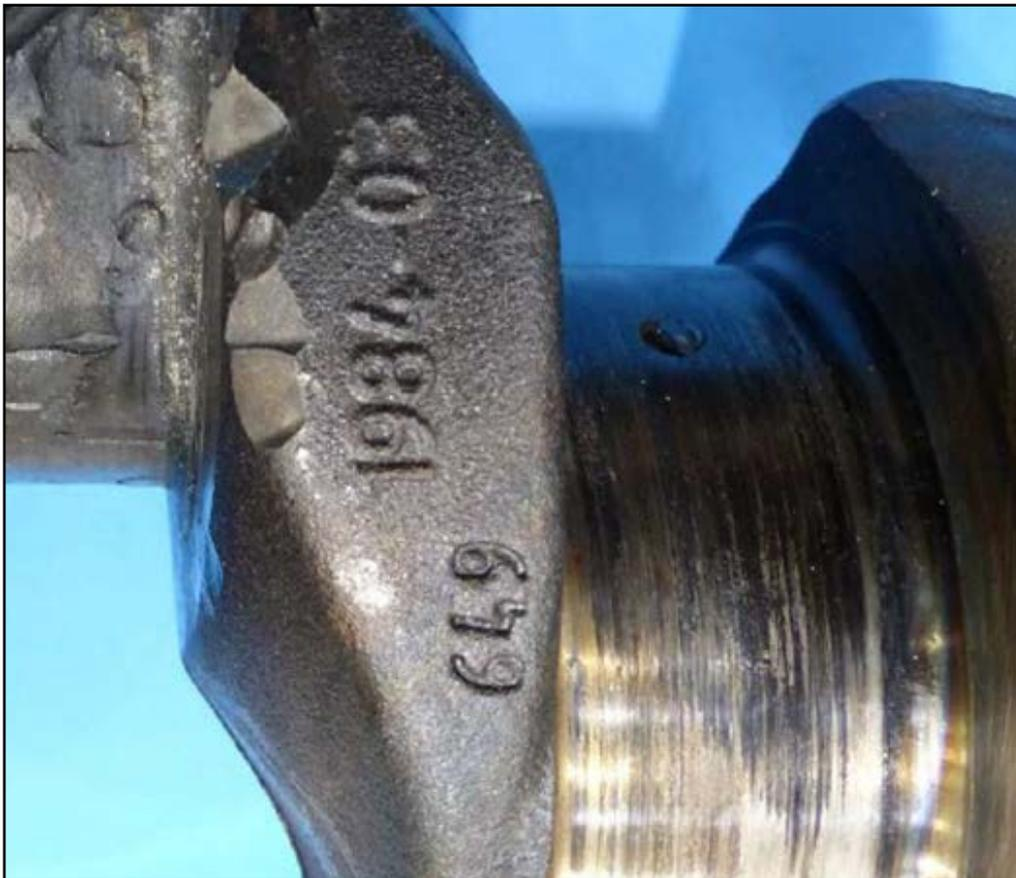
**Figure 25:** Event 4 – heat damage to number four crankpin journal
