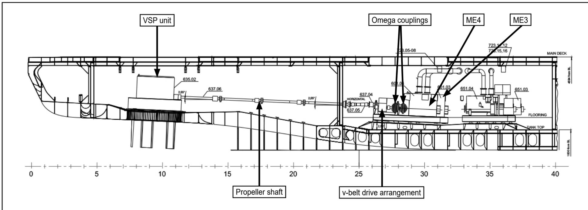
Figure 11: Propulsion system layout
