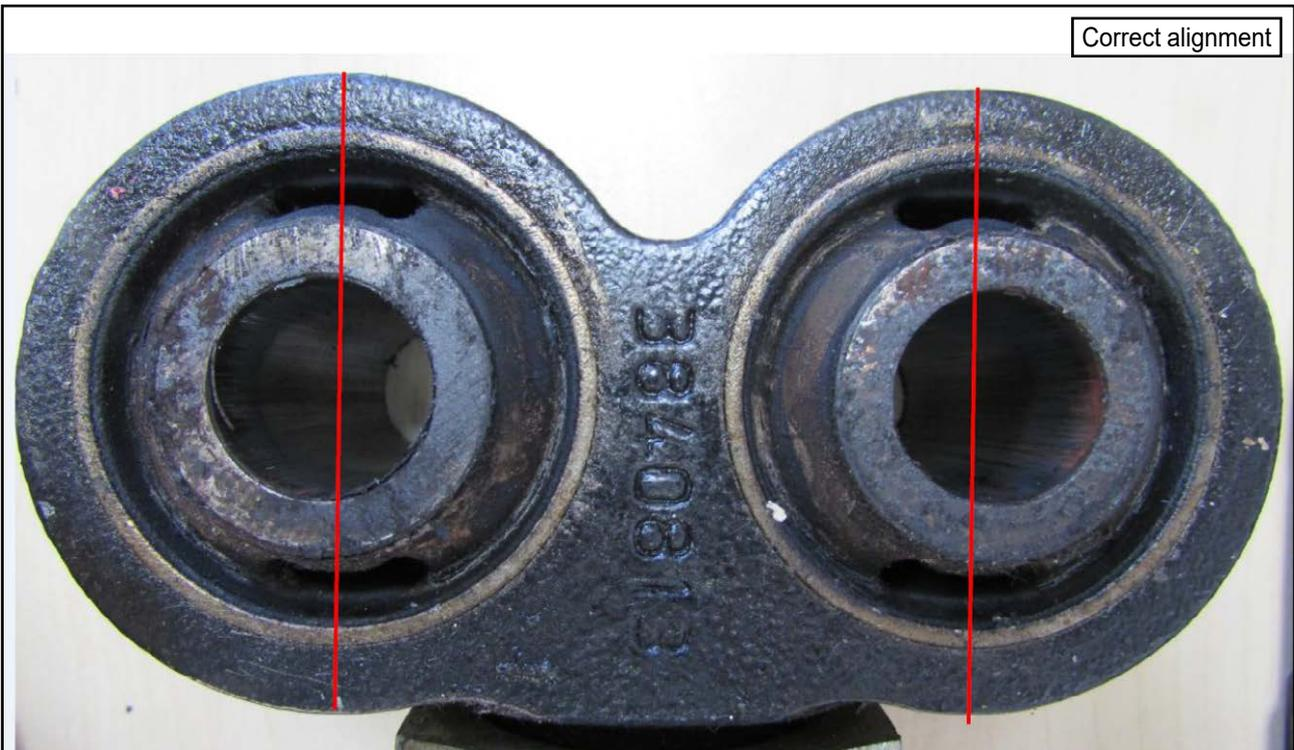
Figure 28: Engine flexible mount rubber bush misalignment
