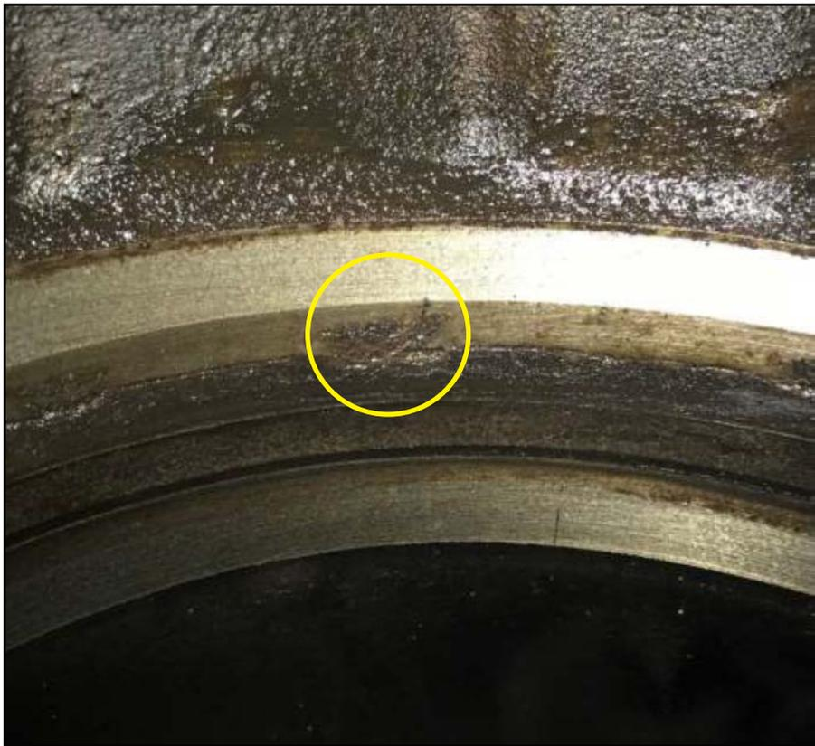
**Figure 30:** Erosion to engine block in line with and below the upper of the two lower cylinder liner seals
