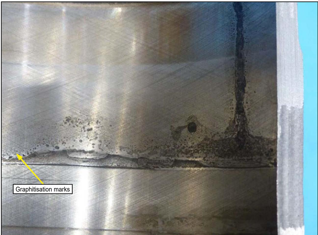
**Figure 27:** Event 4 – graphitisation marks on number four cylinder liner
