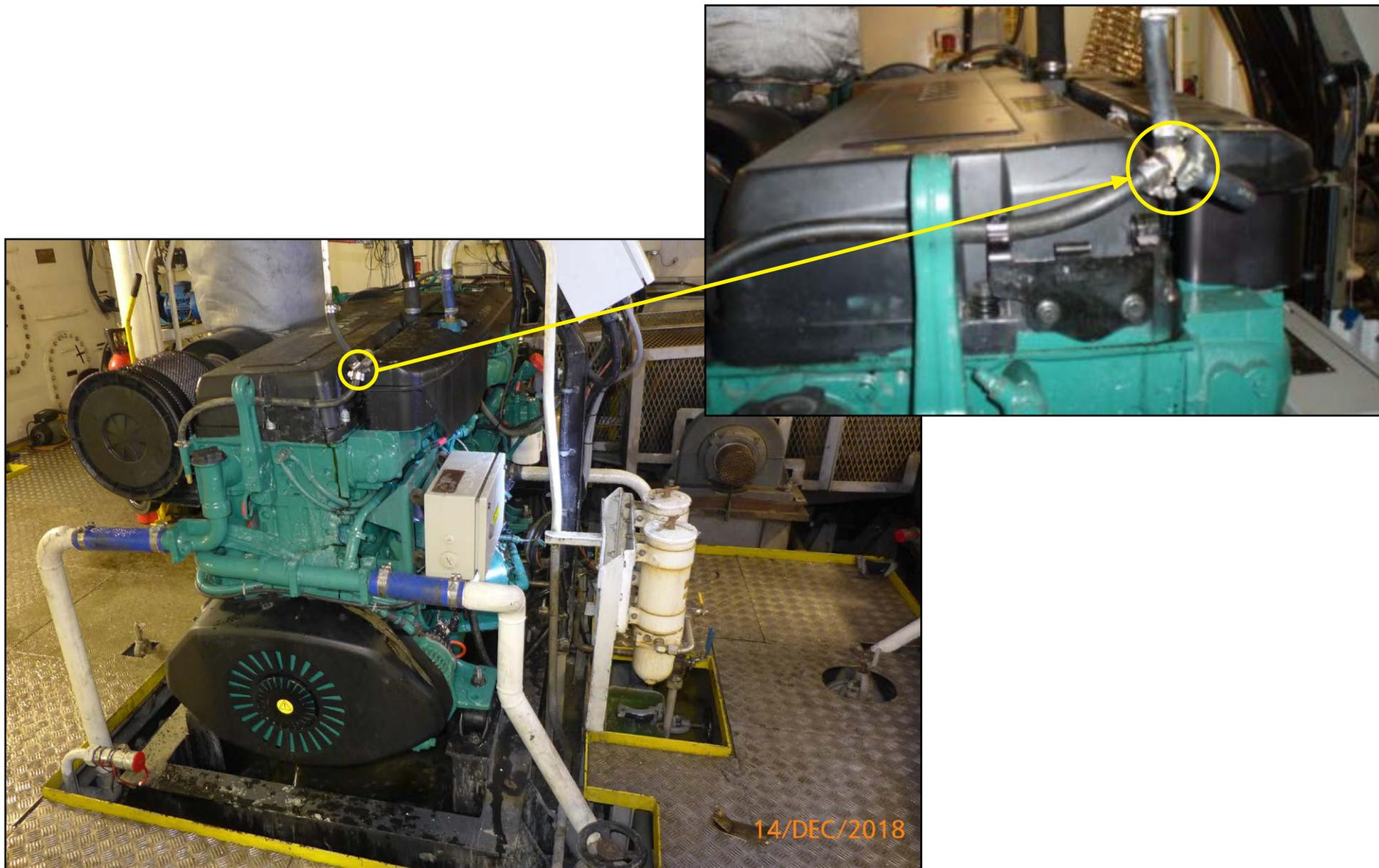
Figure 15: Coolant system T-piece
