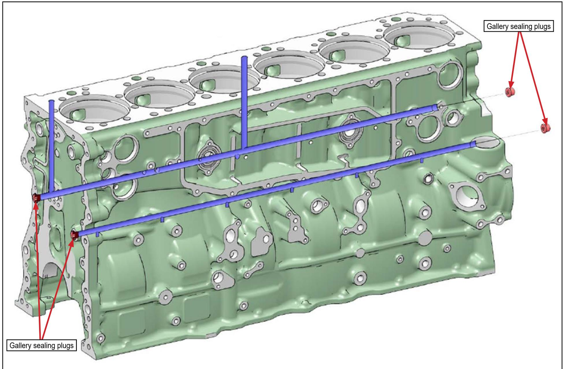
**Figure 18:** Engine block lubricating oil galleries
