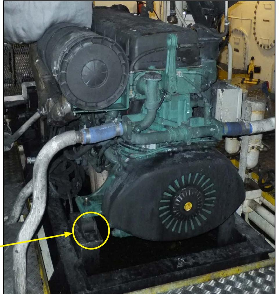
Figure 13: Flexible engine mounts
