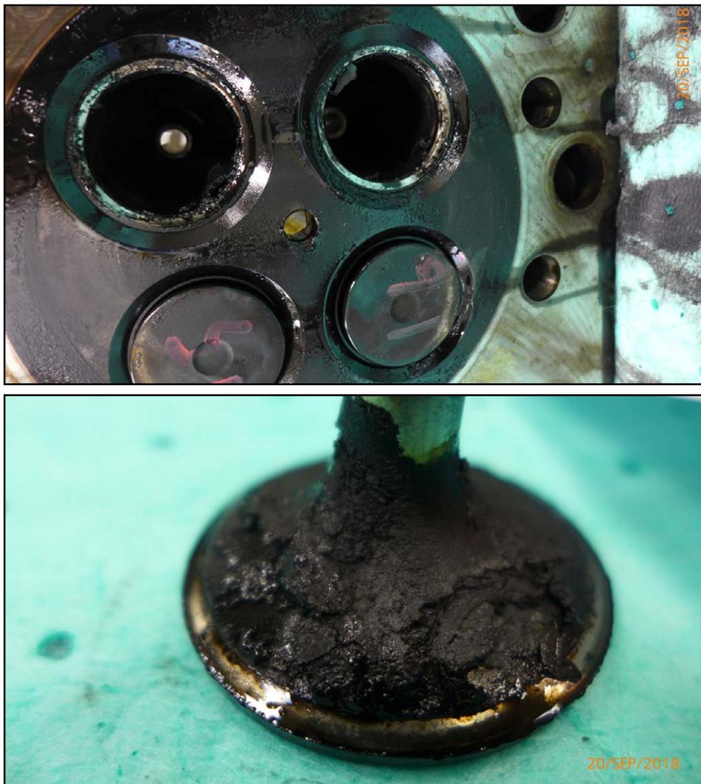
**Figure 24:** Event 4 – carbon deposits on cylinder head valves
