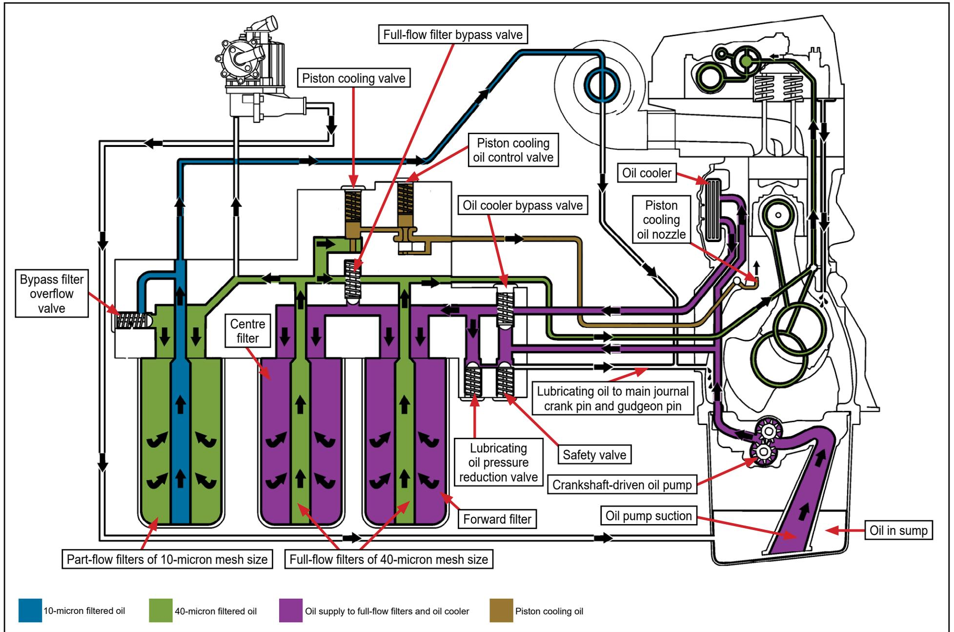
Figure 17: Engine lubricating oil system
