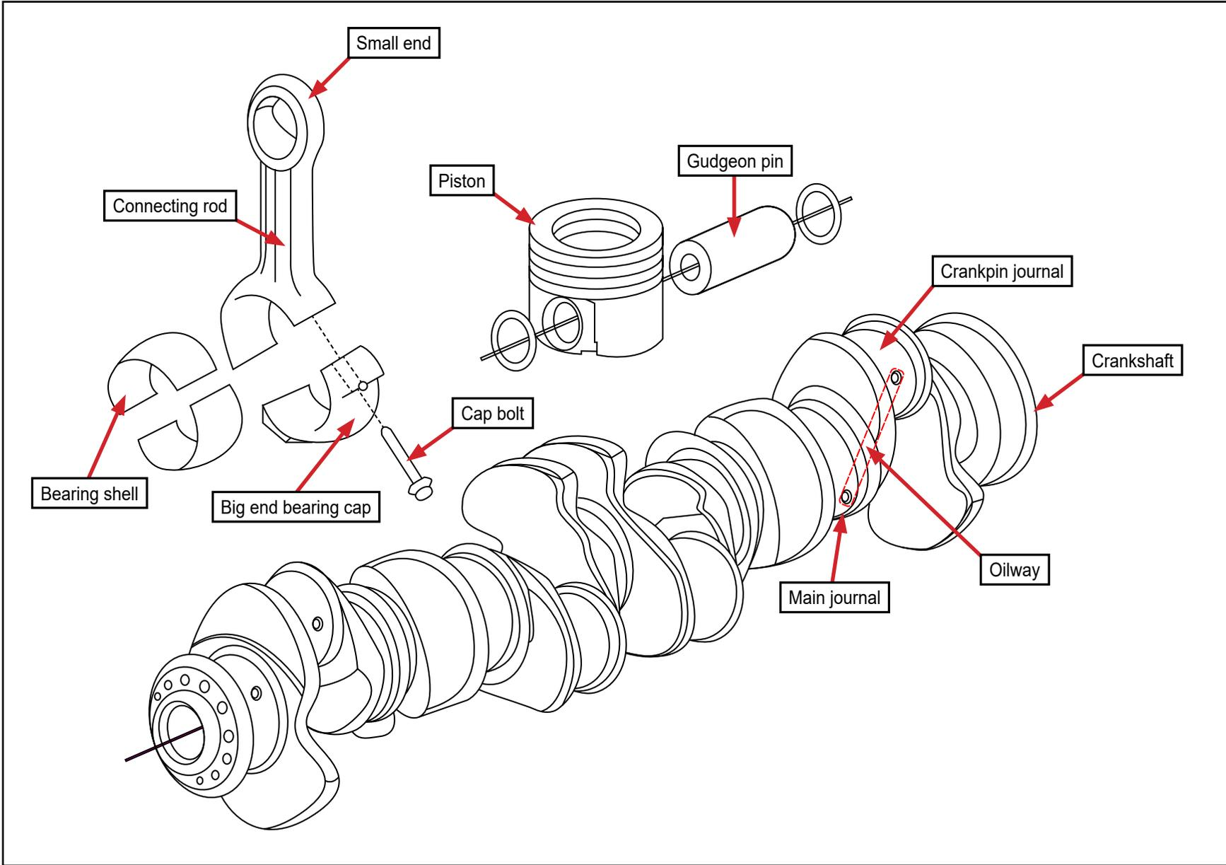
Figure 9: Schematic of rotating assembly
