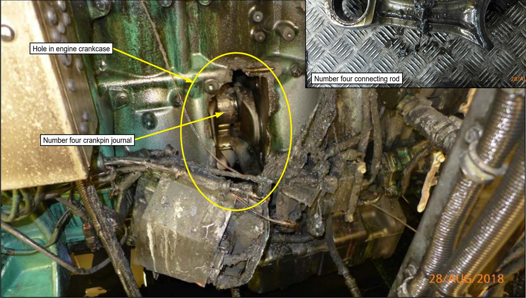
**Figure 4:** Hole in ME2 crankcase, showing number four crankpin journal, and inset, showing number four connecting rod on the engine room deck plate
