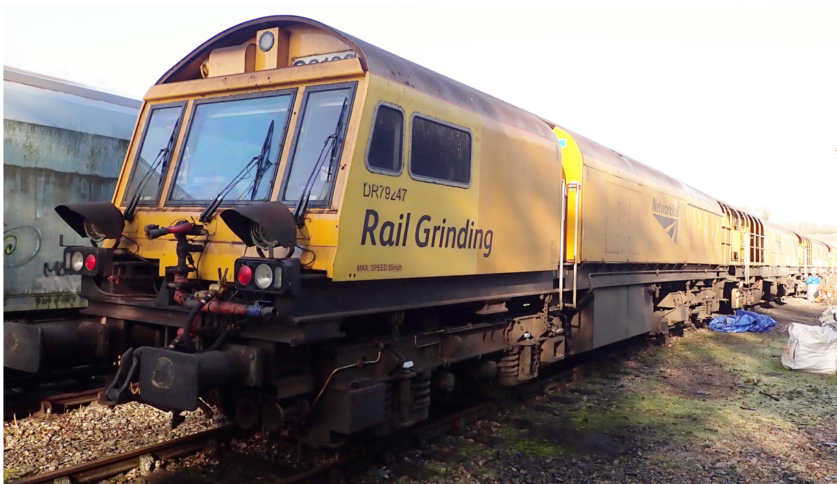
Figure 4: Rail grinding train similar to C2101
