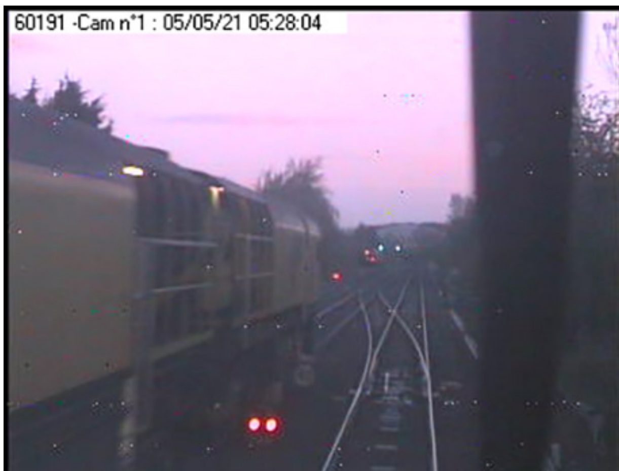
Figure 2: Still image from the rearward facing closed-circuit television (CCTV) of train 5P01 having just crossed over from the up fast line to the up slow line, across the path of train 6Z08; image shows the leading end of rail grinding train 6Z08 (left) shortly before it came to a stop on the down slow line (East Midlands Railway)
