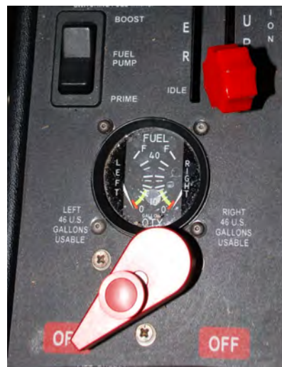
Fuel selector valve, fuel gauge and fuel pump switch
