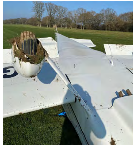
Contamination and damage to one of the wheel spats (pictures courtesy of the pilot)
