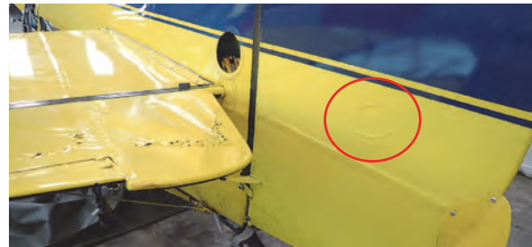
Elevator and rudder damage (circled)
