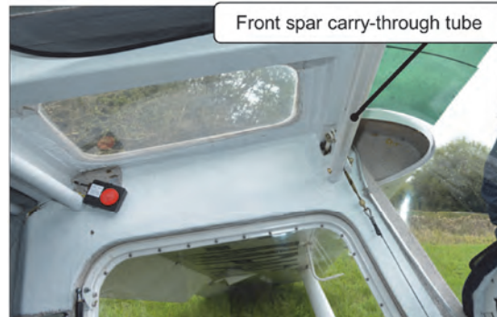
Front spar carry-through tube crossing behind G-MPAC's windscreen (image © Leicestershire Police)
