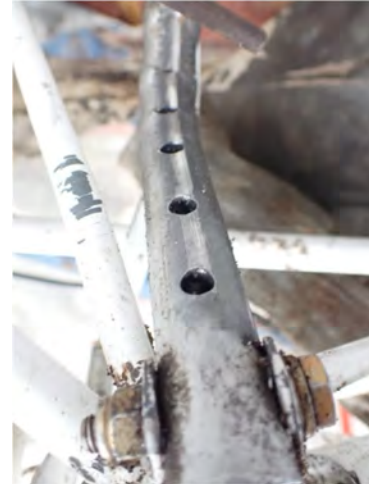
Marks created on the pilot's seat adjustment rail by the pin
