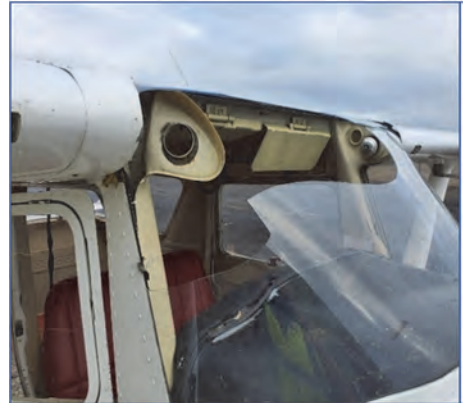
Aircraft damage caused by the impact with the ground
