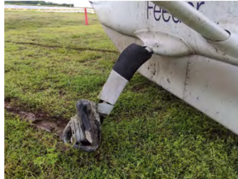
Damage to right wheel assembly
