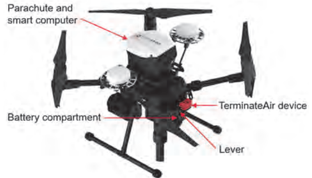
Parazero SafeAir M200 installed on a DJI Matrice 210 RTK unmanned aircraft (Source: Parazero)
