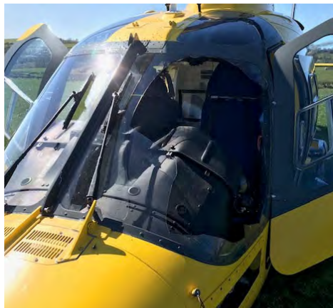
Damage to the left windshield
