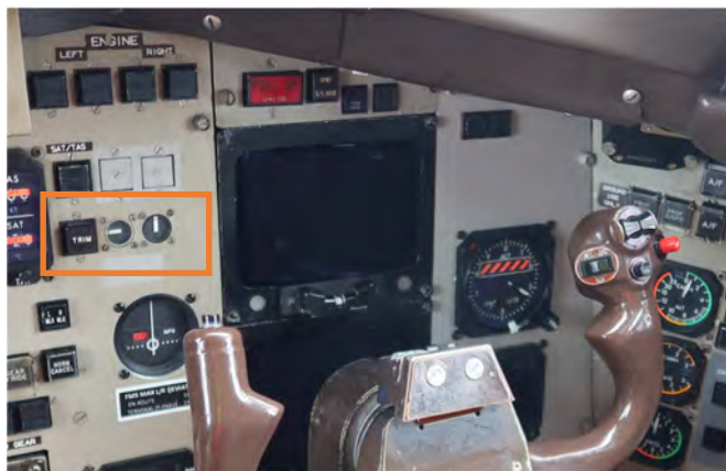
trim light and associated pitch and roll out-of-trim indicators (highlighted in the orange box)
