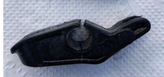
Plastic fuel pump rocker arm
