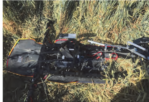
UA as found (inverted) at the accident site
