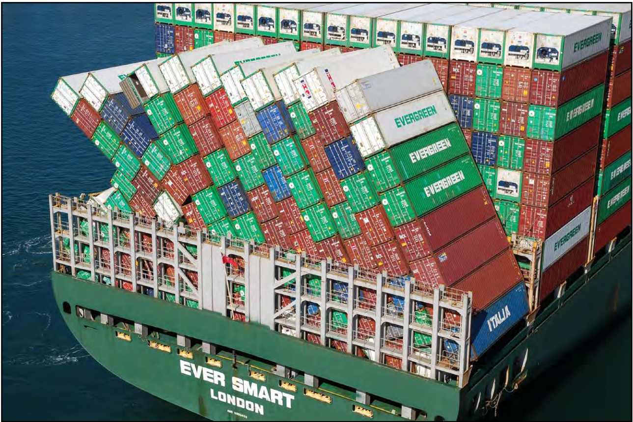
Figure 3: Bay 70 container stow collapse to port
