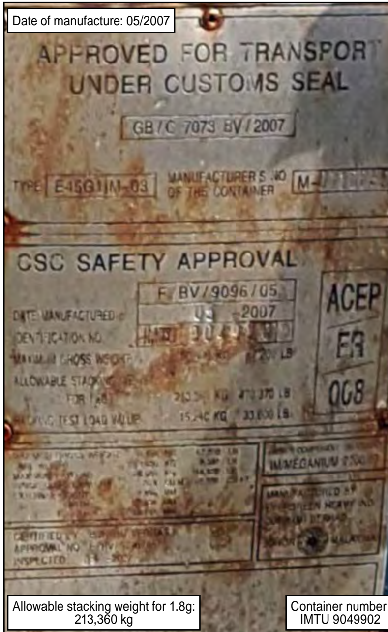
Figure 26: CSC plate and Classification Society approval certificate for the container stowed at the bottom of Bay 70's starboard outer stack
