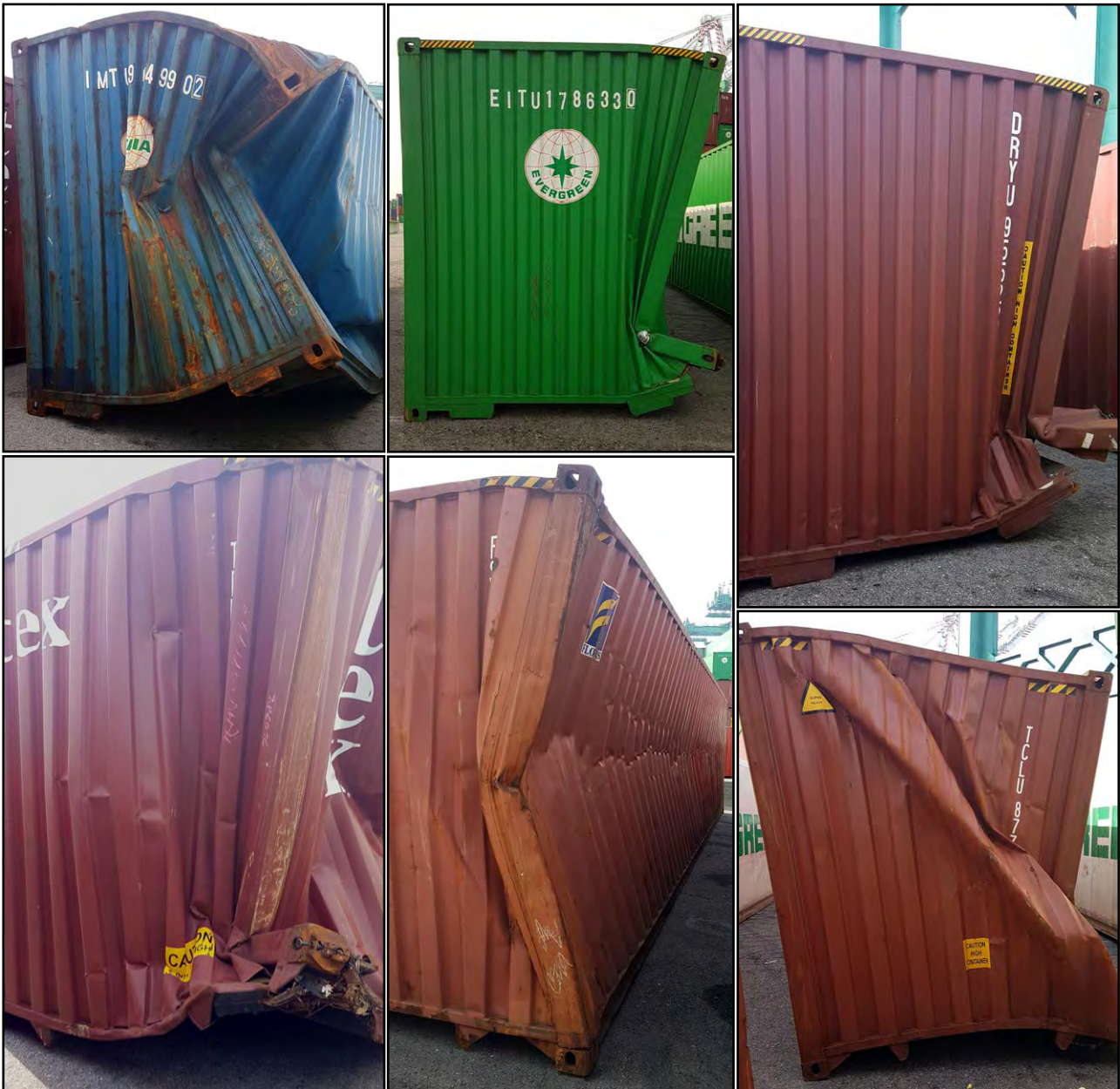
Figure 21: Damage to port forward corner posts of the containers stowed in Bay 70, tiers 1 and 2
