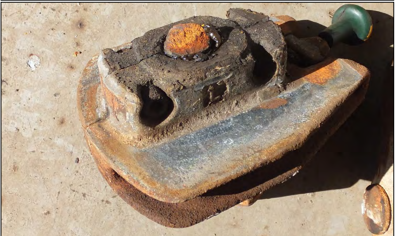
Figure 18: Bent and damaged turnbuckles, lashing rods and twistlocks
