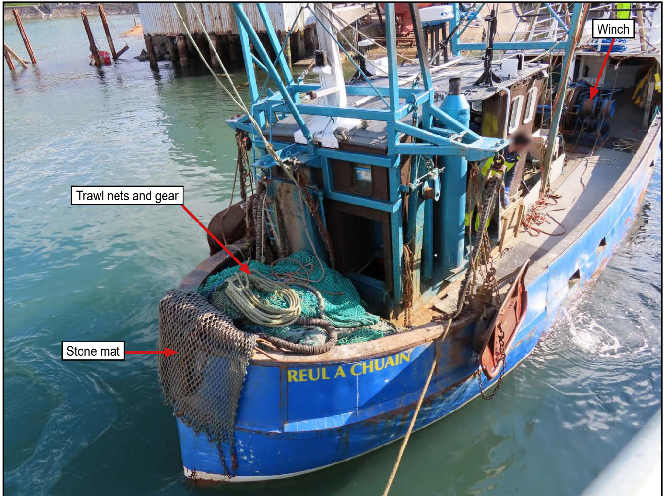
Figure 2: Nets stowed at stern (post-accident)
