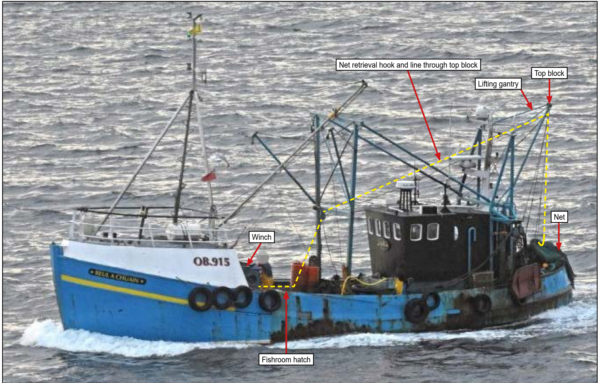
Figure 4: Diagram of net retrieval hook rig
