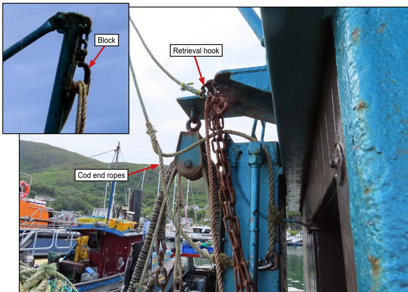
Figure 3: Net retrieval hook, block, and cod end ropes
