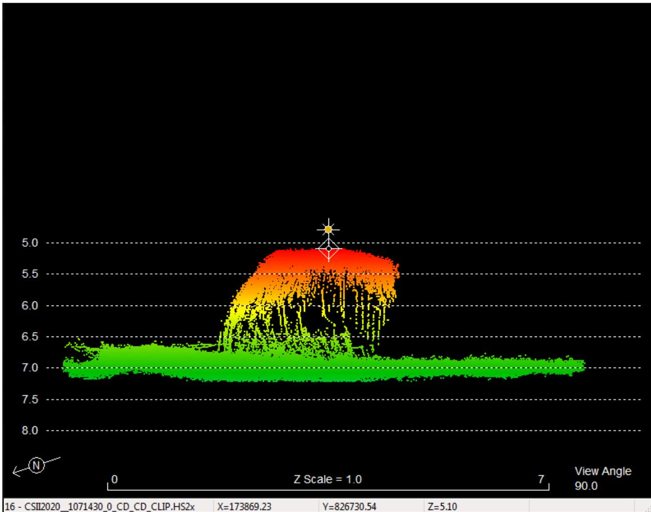
**Figure 12:** MBES image of the 4.9m boulder in the grounding position
