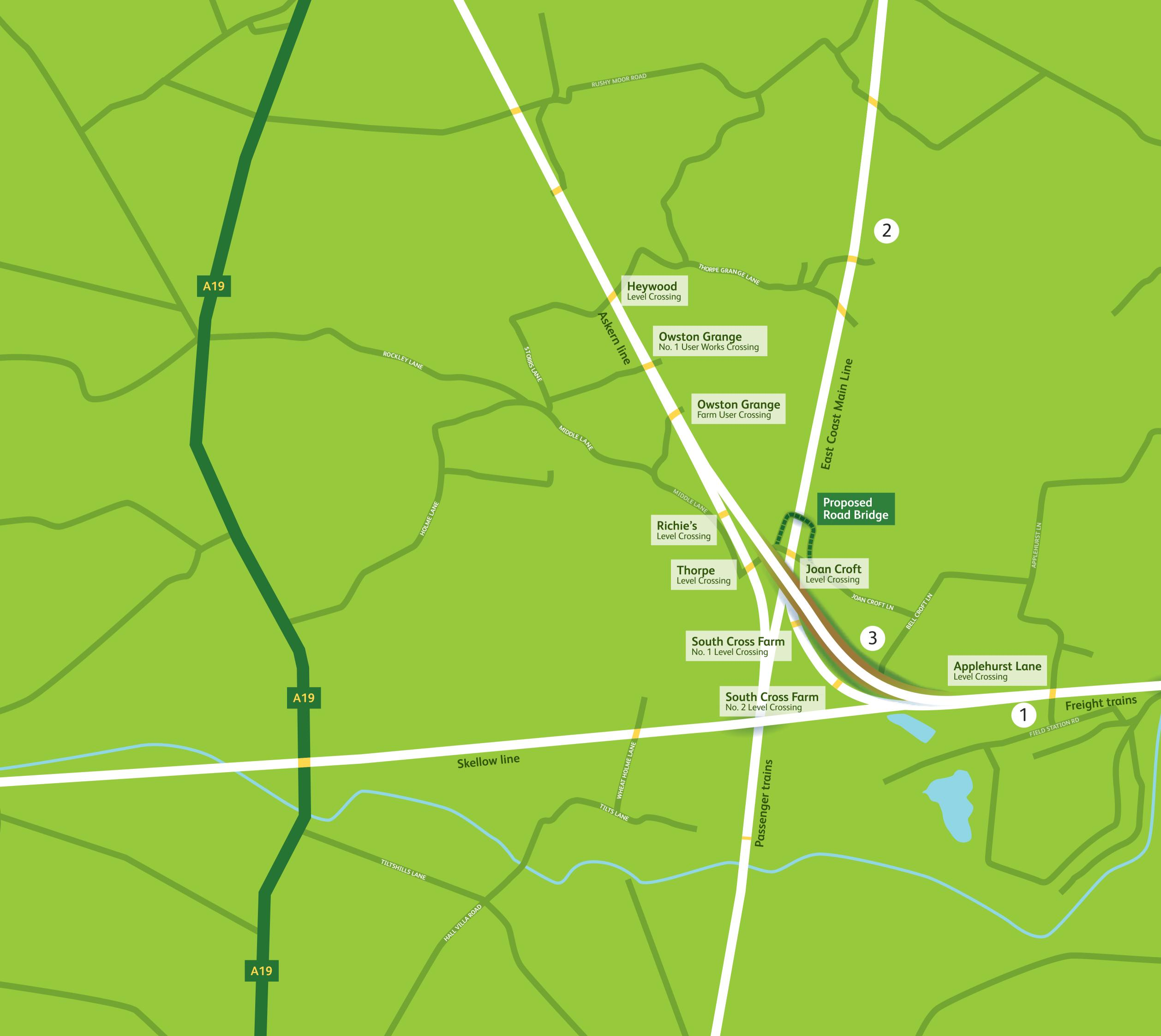
Freight trains travel on Skellow line, on to Applehurst chord and then onto the East Coast Main line (ECML). 2 Freight trains rejoin the Askern line via Temple Hirst junction (12 miles up the ECML). Proposed new track. 3 This would remove the
