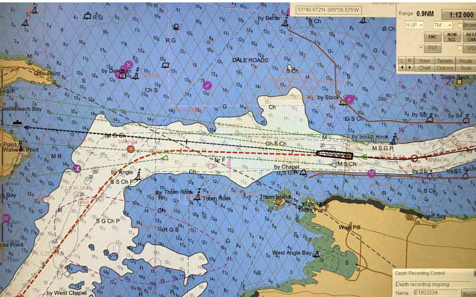
Figure 7: Absence of danger lines or no-go areas
