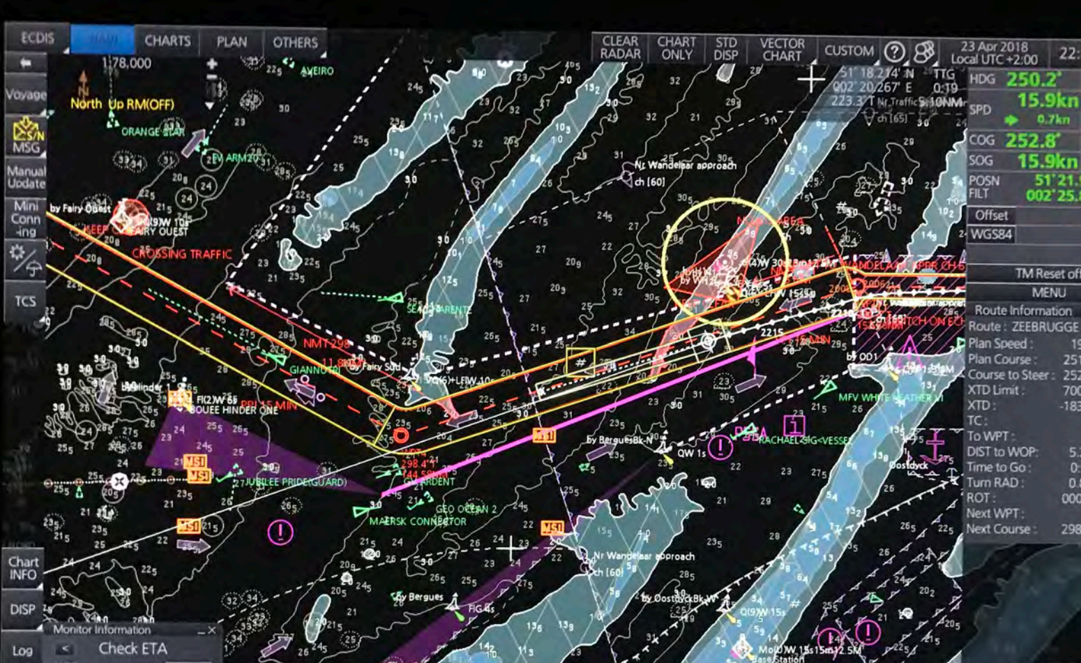
Figure 19: AIS overlaid on ECDIS display
