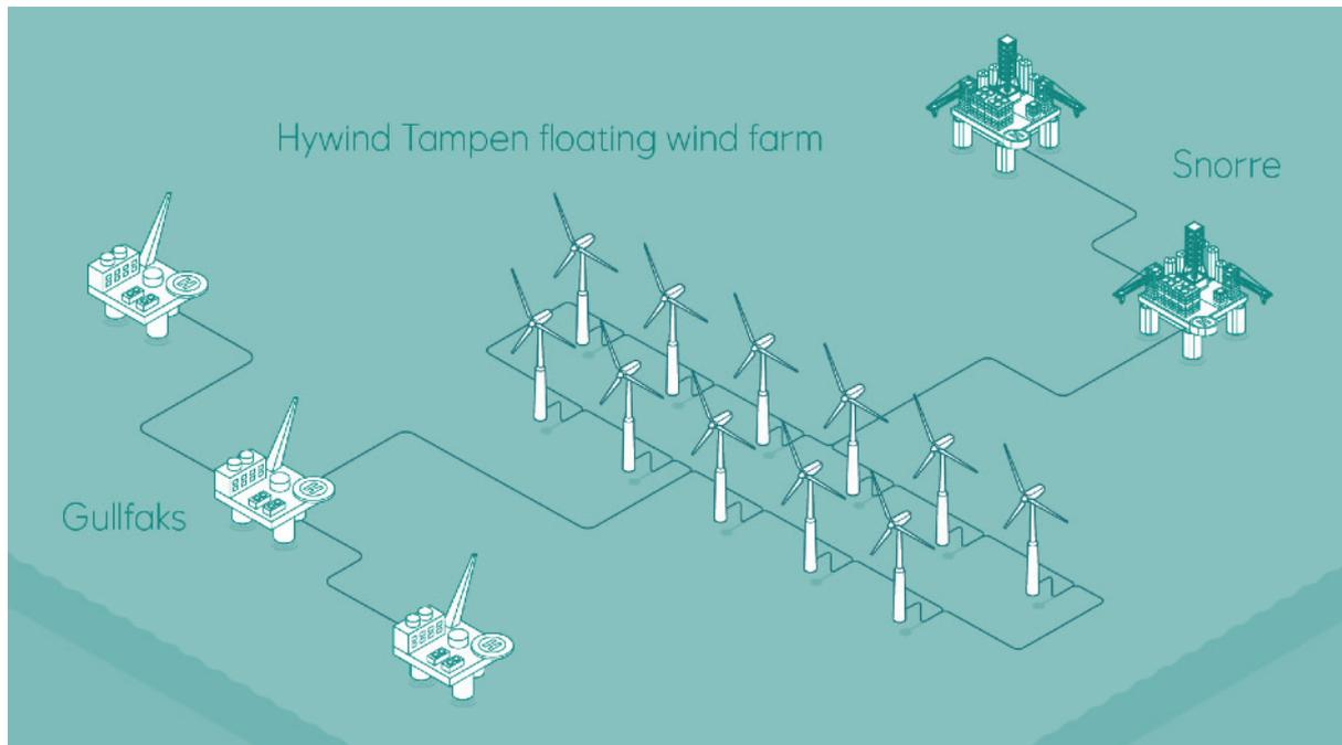
Equinor is moving strategically into the floating offshore wind business with the aim of building a strong offshore wind portfolio, whilst also using offshore wind farms to reduce the carbon footprint of their existing oil and gas activities. Floating wind turbines, relative to bottom fixed turbines, are still in a relatively early stage of development, but Equinor is continuously working on optimizing and opening up new markets for the technology.
