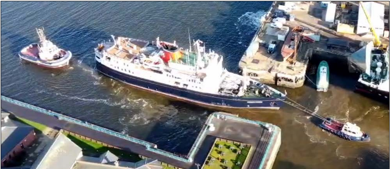
Figure 1: Hebridean Princess leaving James Watt Dock on the morning of 24 February 2023, assisted by the conventional tug Biter forward and the azimuth stern drive tug Wrestler aft
