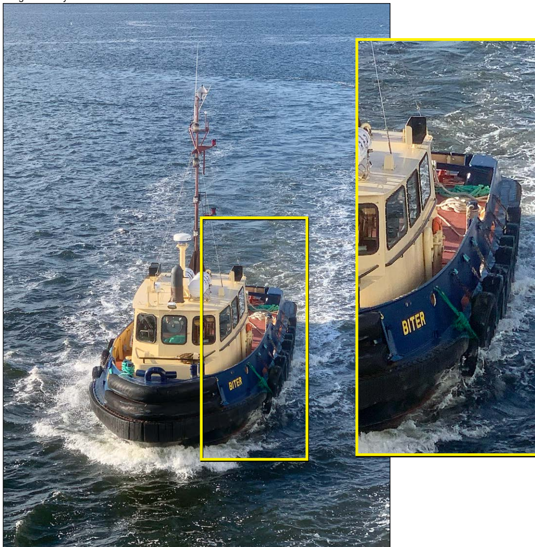
Figure 4: Biter running alongside Hebridean Princess's starboard quarter, before the lines were passed, showing the tug's gob rope secured to the port side samson post
