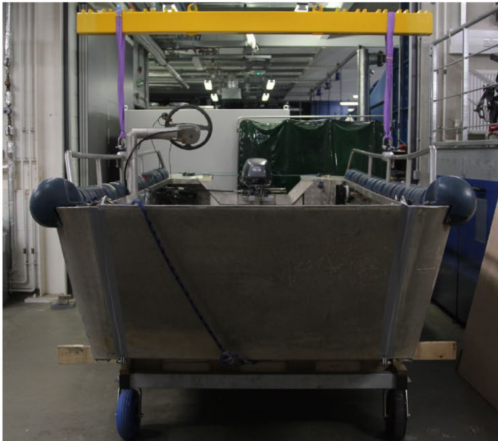
Figure 4 Inclining experiment rig
