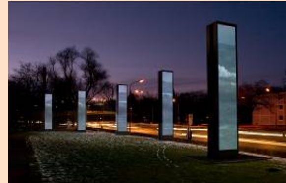
The art project SEVEN SCREENS at OSRAM headquarters in Munich – a project developed in cooperation with OSRAM Light Consulting - shows that the OSRAM brand is 104 years young. 700,000 high-power RGB LEDs (16 mio different colours possible) have been installed on the masts and can be controlled via fibre optic cable from a central computer room.
